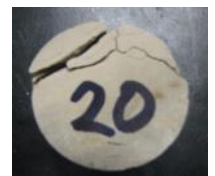
1 1/2" Carbonate plug Porosity = 18.9%
