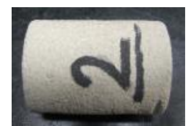
1 1/2" Sandstone plug Porosity = 22.5% Permeability = 158mD
